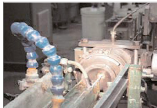
Extruding of outer sheath
