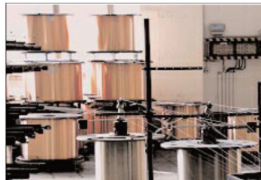
Stranding of single wires
